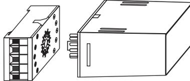
picture 2: Horizontal mounting orientation, ventilation slots top
