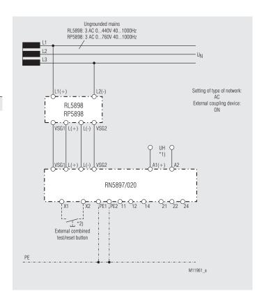
$^{\ast}1)$  Auxiliary voltage  $U_{_{\rm H}}$  (A1(+)/A2) ) can also be sourced from the monitored voltage system.
