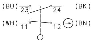
The colour allocation refers to the plug-in-cables which we have in our range.
